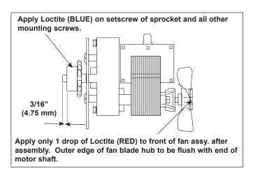
Figure 11. Replacing Drive Motor and Fan Blade
